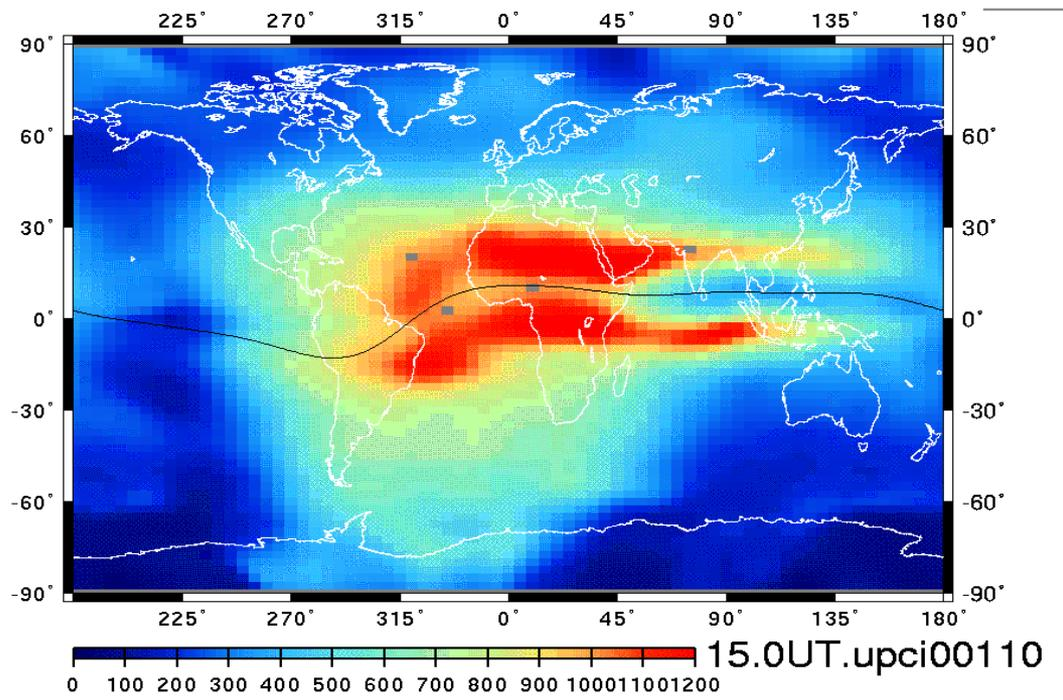
Global Vertical Total Electron Content (VTEC) map computed from ~100 GPS dual-freq CORS (units: 0.1 TECU).[\*]
