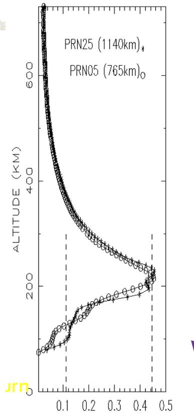
Electron density (Ne) profile computed from LEO GPS data (units: Te-/m<sup>3</sup>).[\*]
