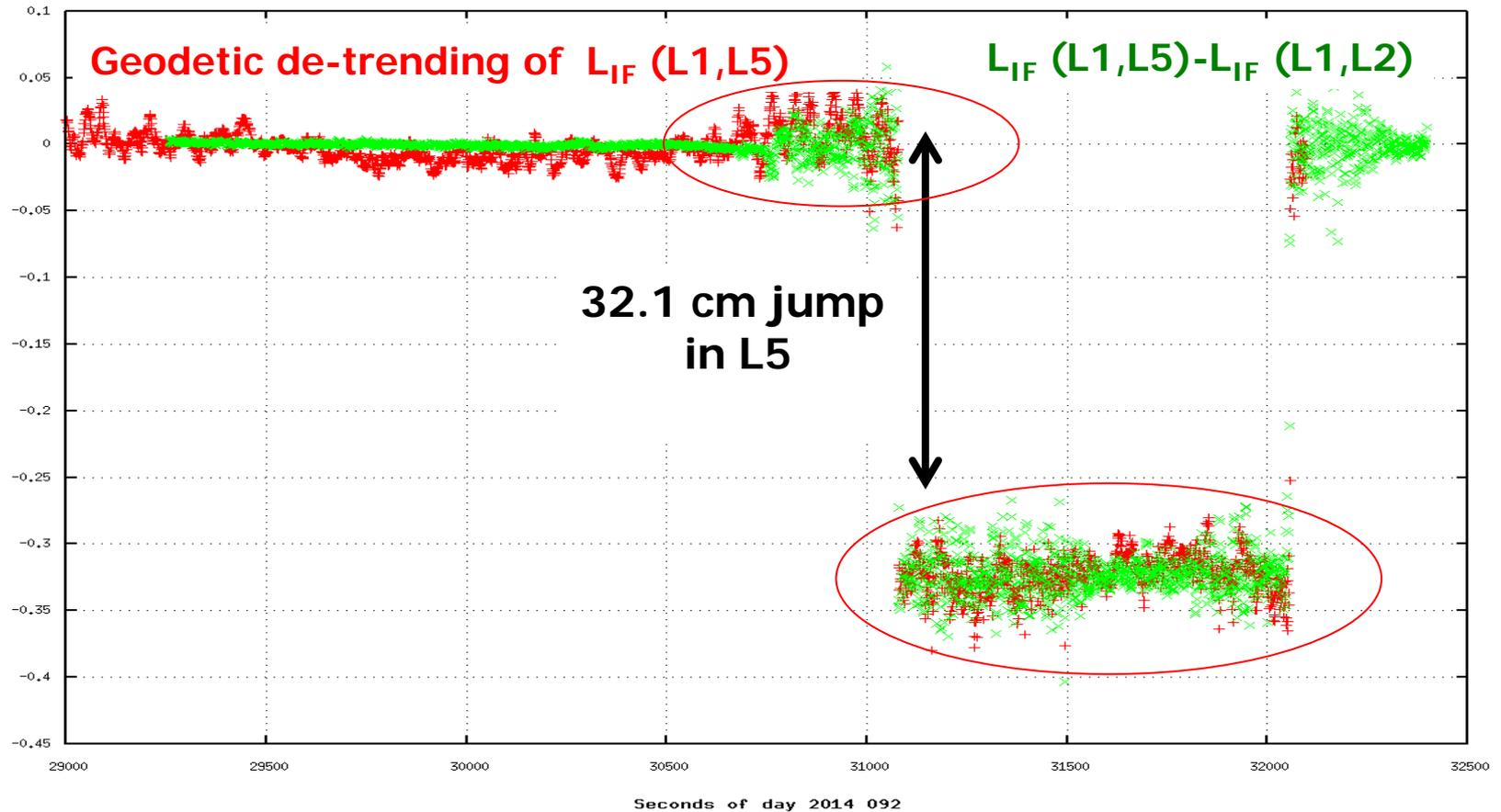
With three frequency systems, the combination geometry-free and Ionosphere-Free can be explored as **a real-time** reliable detector of 1-cycle jumps.
