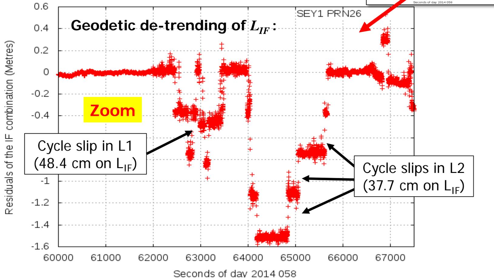
With a geodetic de-trending of  $L_{IF}$ , it is possible to distinguish between these 1-cycle jumps occurring in L1 (0.484 m) and L2 (0.377 m)
