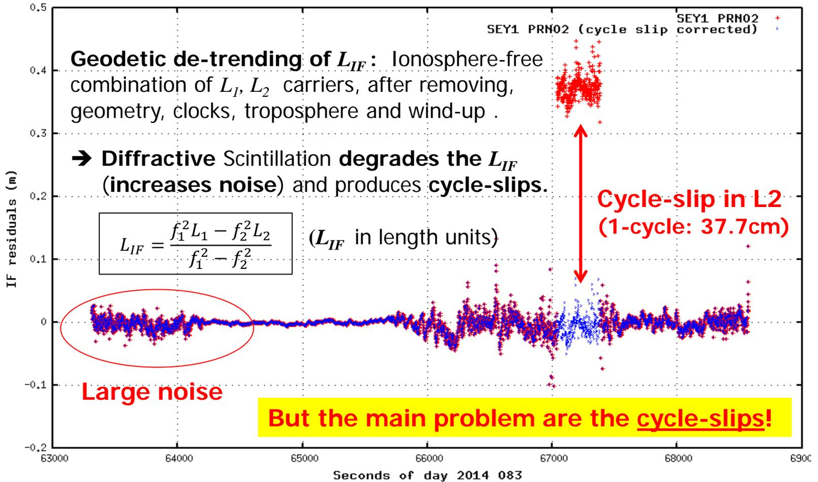
The geodetic de-trending of  $L_{IF}$  allows to depict the increased noise and the 1-cycle jump.
